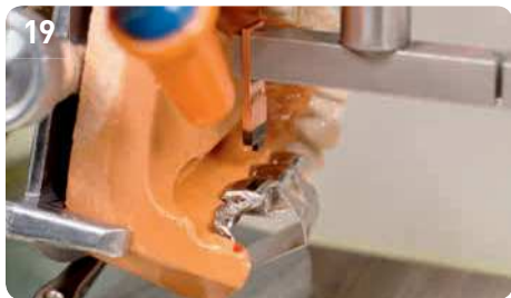
The spark erosion process is complete when the set depth is reached, erosion time approx. 20 minutes (CoCrMo).
