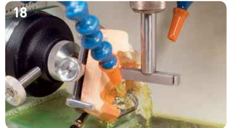
The spark erosion process begins with flushing through the dielectric fluid.
