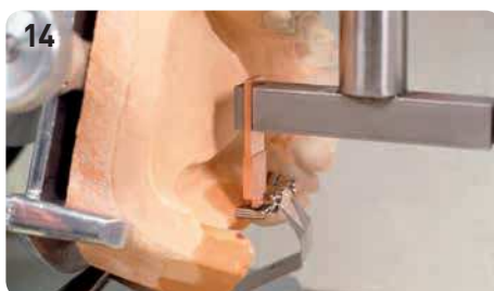
Using the electrode (Order No. 30-1384), the erosion depth is set on the cone of the primary part. The clasp serves to secure the primary part.
