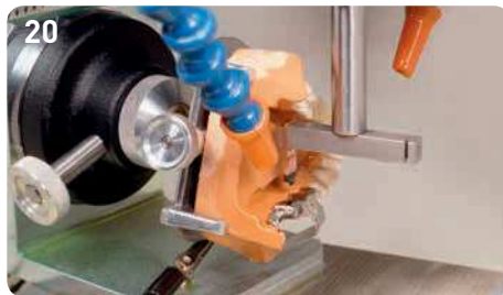
The spark erosion process is complete when the set depth is reached, erosion time approx. 20 minutes (CoCrMo).
