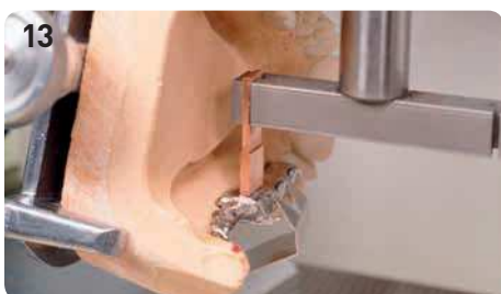
Position the model with the primary-secondary structure. The erosion position is determined by lowering the cut-to-size electrode.
