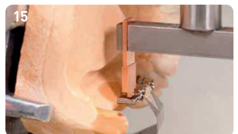
Optical control of the electrode position. The electrode should be lowered towards the cone so that the latch nose slots completely into the eroded groove of the tapered cone.
